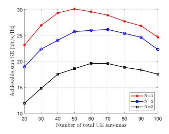
Fig. 8: Sum SE against the number of total UE antennas for Level 2 with MR combining over M = 40, K = 20 and L = 2.
