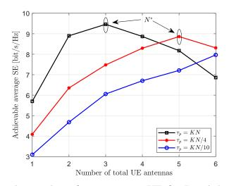
Fig. 7: Average SE against the number of antennas per UE for Level 4 with MMSE combining over different  $\tau_p$  with M = 40, K = 20 and L = 4.
