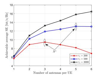
Fig. 6: Average SE against the number of antennas per UE for Level 4 with MMSE combining over different  $\tau_c$  with M = 40, K = 20 and L = 4.
