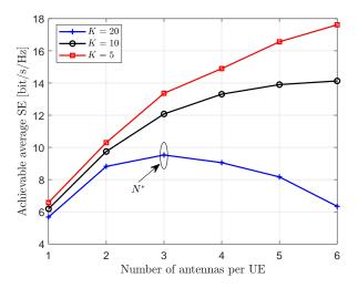
Fig. 9: Average SE for Level 4 over MMSE combining as a function of N with M = 40, K = [5, 10, 20] and L = 4.
