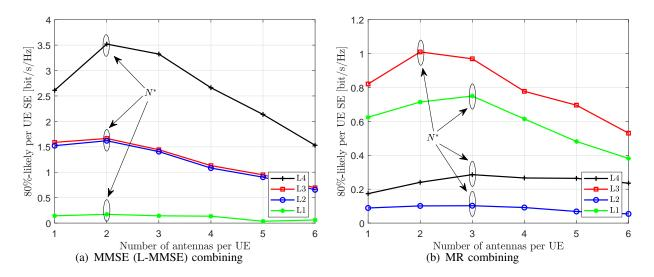
Fig. 5: 80%-likely per-user SE for MMSE (L-MMSE) combining and MR combining as a function of N with M = 40, K = 20 and L = 4.
