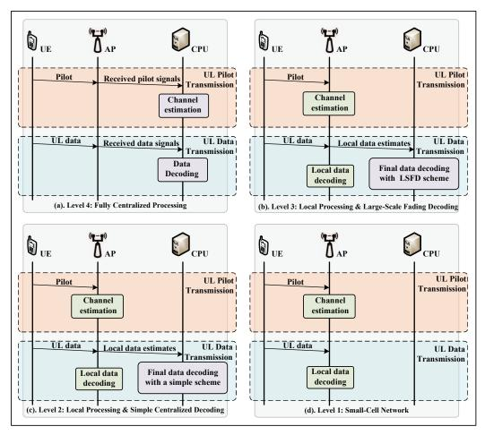
Fig. 3: The comparison of four UL implementations.
