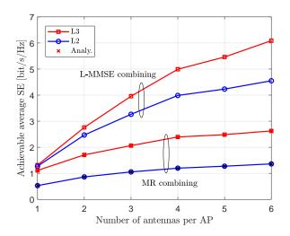
Fig. 11: Average SE against the number of antennas per AP for Level 3 and Level 2 over L-MMSE combining and MR combining with M = 40, K = 20, N = 2 and  $\tau_p = KN/2$ .
