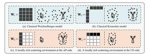
Fig. 2: Different structures of the coupling matrix and respective physical radio environments.
