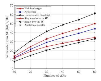
Fig. 10: Sum SE against the number of APs for Level 3 over MR combining and different channel models with K = 10, L = 4, N = 4 and  $\tau_p = KN/2$ .
