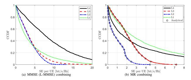
Fig. 4: CCDF of SE per UE for MMSE (L-MMSE) combining and MR combining with M = 40, K = 20 and L = 4.
